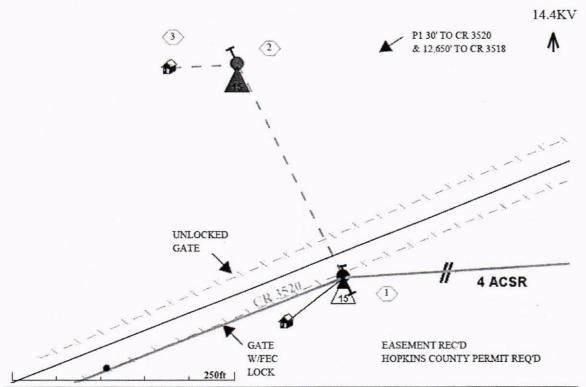
Misc. Remarks: EXTEND OH PRIMARY 1 SPAN ACROSS CR 4762 FROM P#090574, HANG XFMR/CUTOUT, AND DROP OH SERVICE TO 200A OH PMP SERVING 2000SF STL FRAME HOUSE BEING BUILT. 1 EASEMENT REC'D. HOPKINS COUNTY
